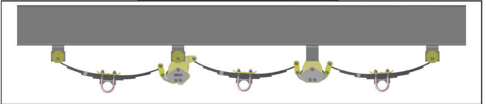
Fig. 5.1 - Triple Axle With Equaflex Installed
