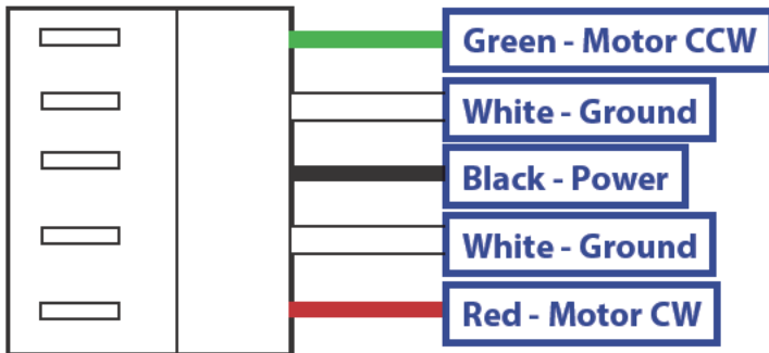
Fig. 1 Old Slideout Switch Color Codes
